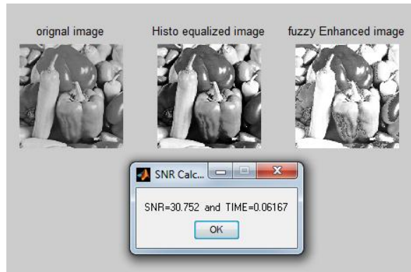
FIGURE 5.4: (A) ORIGINAL IMAGE (PAPPER), ENHANCED IMAGE WITH (B) HISTOGRAM EQUALIZATION (C) PROPOSED METHOD WITH SNR AND TIME CALCULATION.
